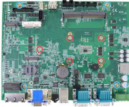
Securing the motherboard
